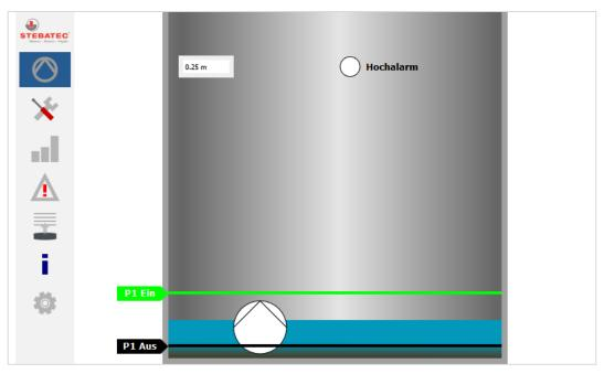
Figure 2: Visualisation of pump control on the zoomable touch panel, whereby, depending on the configuration, several pumps and other components such as exhaust air system etc. are displayed.
