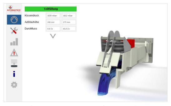
Figure 3: View of ALLinONE panel with integrated control of a rainwater basin's discharge control.
