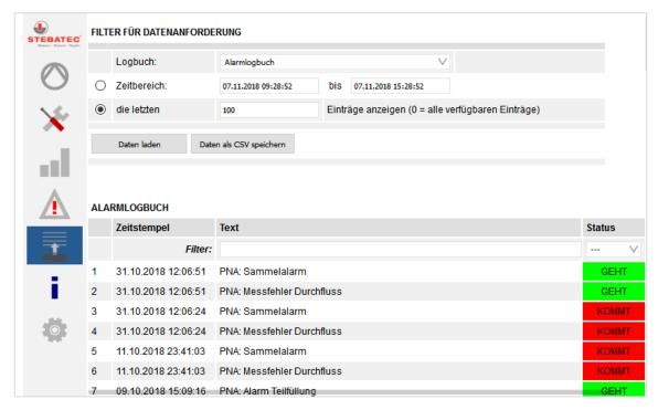
Figure 5: Alarm list of the ALLinONE system, with the possibility of searching for specific alarms with the filter or exporting the list.
