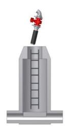
Place «Portable» upright Lower it on ropes Do not pull the cable/hose
