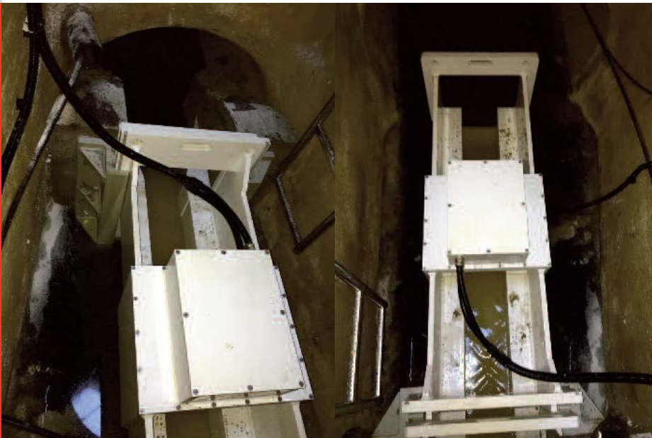
The part-filled stationary flow measurement of the Steg measuring station at low flow rate (dry bed only).
