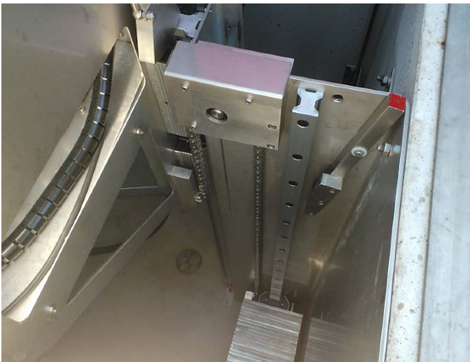
Lifting mechanism with counterweights (bottom) and locking lever (right).
