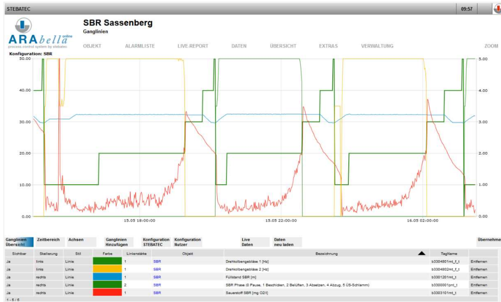
Figure 4. The graphs represent 3 cycles. The duration of the cycles is not the same for each cycle. The aeration phase is terminated when the oxygen concentration rises above 1.8 mg/l.
